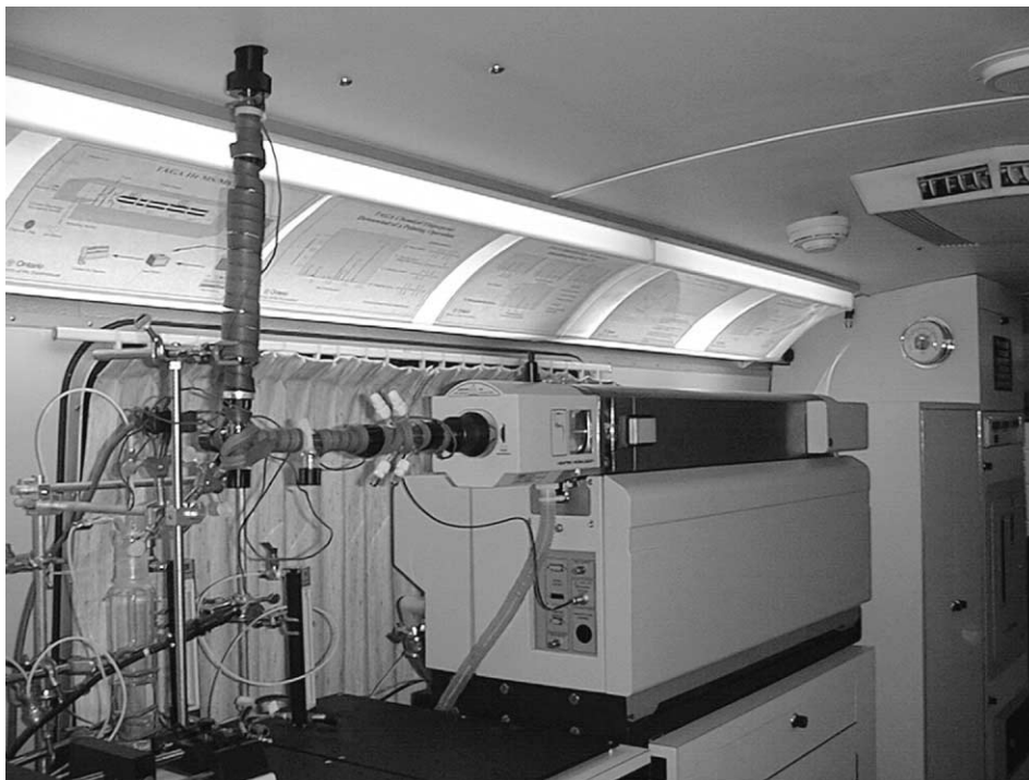
Fig. 2. The TAGA IIe mass spectrometer housed inside the mobile unit, known as the “Explorer”.
